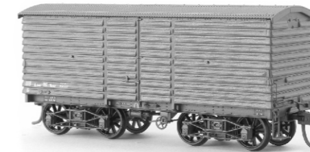
UB van with swing motion diamond frame bogies. 1955 - 1960
