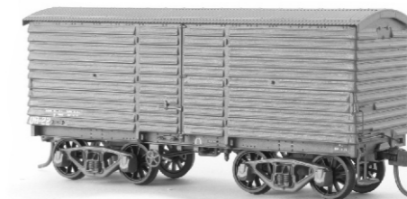
UB with 40 Ton cast steel bogies. 1973 - withdrawal
