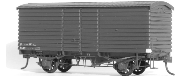
U van with original handbrake rigging.
