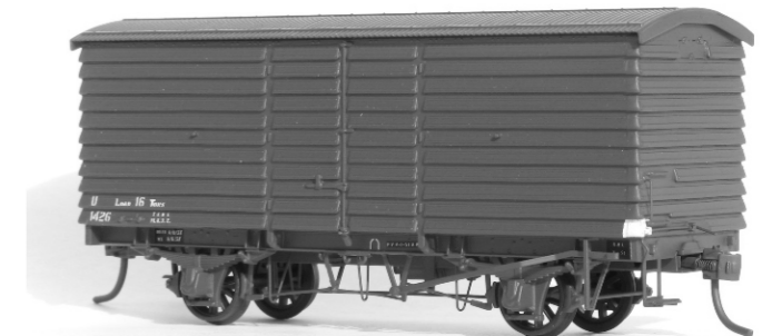
U van with modernised hand brake rigging.
