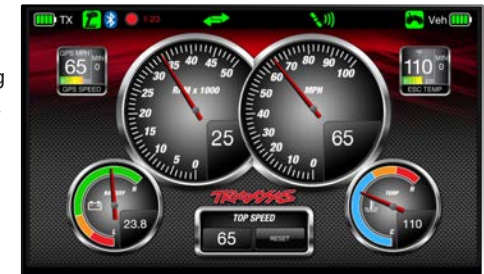
The customizable Traxxas Link dashboard delivers real-time rpm, speed, temperature, and voltage data.
