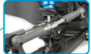
Rugged steel turnbuckles for adjustable camber and front toe-in
