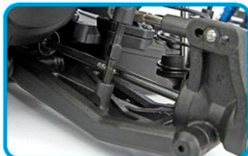
Rear CVA driveshafts for more reliability
