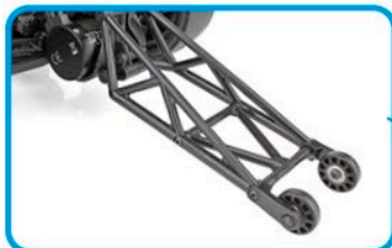
Three-position wheelie bar with optional large wheels included
