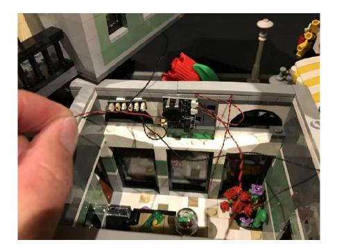
27.) We will now test the lights we have installed so far as well as adjust the speed of the flicker effect for the fountain. Take the battery pack and connect the battery pack cable into any of the spare ports of one of the expansion boards. Turn on to verify all is working ok.
