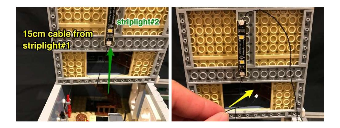
Reconnect the third level on top and then pull the connecting cable up from underneath ensuring it is threaded behind the staircase.
