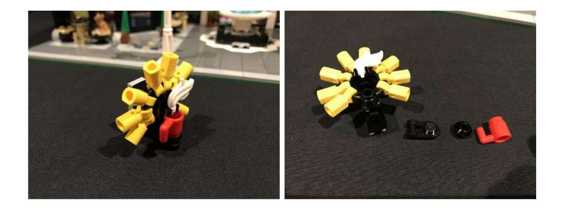
Take a bit light with 15cm cable and place the LED component directly over the stud of the black piece. With the cable facing toward the back, reconnect the round black piece directly over the top to secure the bit light in place then thread the cable down underneath the space of the black LEGO piece
