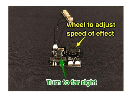
24.) Using another 2 adhesive squares for each, mount the 2 different boards to the inside wall of the flower shop and connect the 15cm cable from expansion board in the patisserie into the first available port of the 6-port expansion board as per below:
