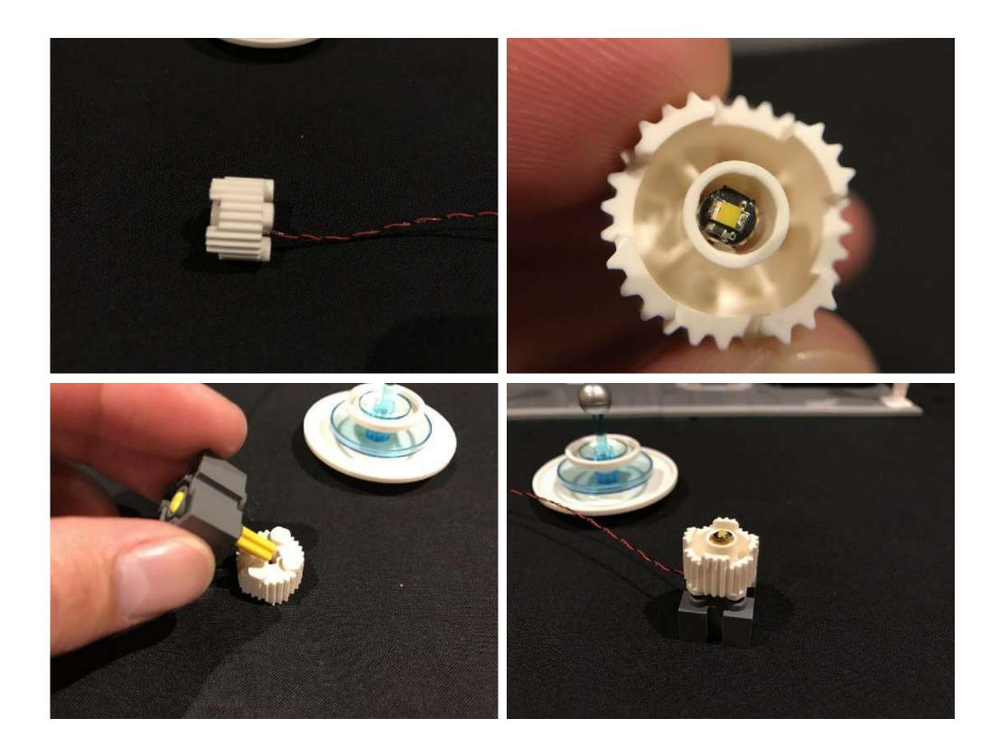
Note: Because of the bit light cable. the 2 sections (white round brick and dark grey brick) will not fully connect and there should be a slight 1-2 mm gap between the two.
