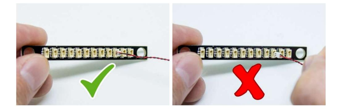
**Installing Bit Lights under LEGO® bricks and plates.** When installing Bit Lights under LEGO® pieces, ensure they are placed the correct way up (Yellow LED component exposed). You can either place them directly on top of LEGO<sup>®</sup> studs or in between.
