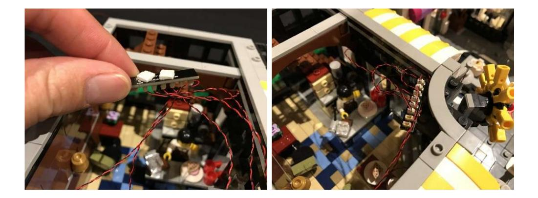
15.) Take a **30cm connecting cable** and connect it to one of the spare ports on the expansion board. Take the other end of the cable and
