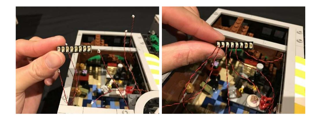
13.) This is a good time to test our current light circuit. To do so, insert 3x AA batteries to the battery pack and then connect the battery pack cable into a spare port of the expansion board. Turn on
