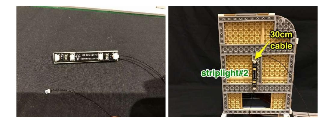
Connect the connecting cable from the level below into the other port on striplight#2 and thread the 30cm cable connected to the other port up the open space which leads to the 3rd level.
