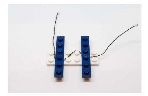
CAUTION: Forcing LEGO® to connect over a cable can result in damaging the cable and light.
