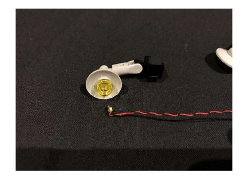
Place the LED component facing upward inside the middle of the trans yellow LEGO piece of one of the lamps. Pull the cable over the
