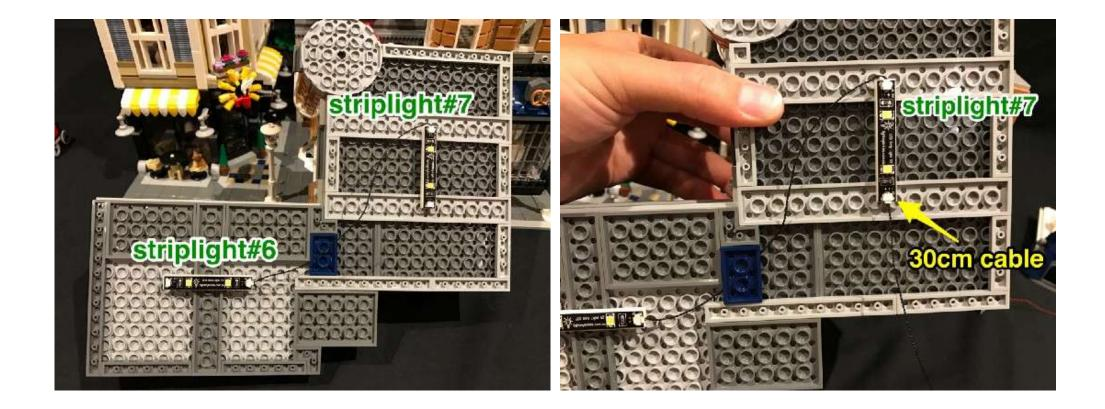
To prevent the cable from hanging down and being seen from the outside looking in, connect LEGO pieces over the top.
