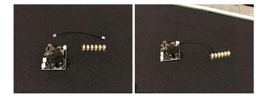
This multi effects board has 3 different effects. For this light kit, we will be using effect# 3 (flicker effect). Set it to the 3rd option by flicking the switch to the far right. We will later use the wheel on the effect board to adjust the speed of the flicker effect as desired.
