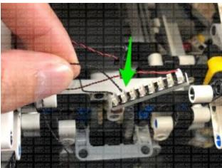
Turn the Battery Pack ON to test the rear Red Strip Light is working OK.
