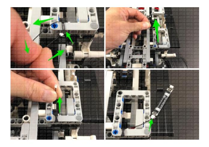
10.) Take a 5cm Connecting Cable and connect it to the other side of the Red Strip Light, then using it's adhesive backing, stick the strip light down vertically on the black technic bar in the below position. Connect the other end of the 5cm Connecting Cable to a new Red Strip Light, then connect a new 30cm Connecting Cable to the strip light's other port.
