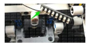
Take the AA Battery Pack and connect the battery pack cable to the 8-Port Expansion Board, then place it inside the trunk. Turn it ON to test all the red strip lights are working OK.
