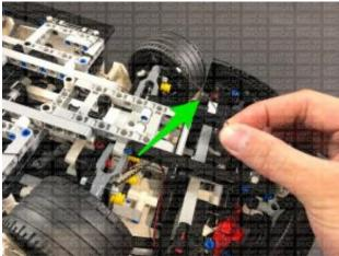
Thread the cable underneath the wheel axis, then through the hole of the grey technic piece as shown below:
