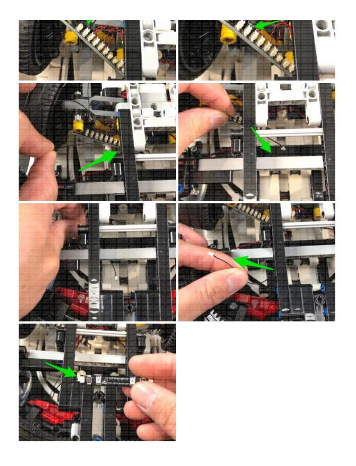
Take a **30cm Connecting Cable** and connect it to the other port on the Red Strip Light. Using the Strip Light's adhesive backing, stick the Strip Light underneath the car in the following position.
