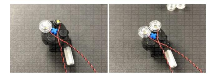
Install another **2x White 15cm Bit Lights** to the two bottom studs as shown below:
