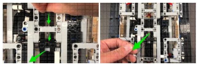
Bring the cable toward the left, underneath the centre bars, then thread the cable through the technic bar hole as shown below. Pull the cable out from the bottom, then bring the cable back over the technic bar and thread it back through the same hole. Connect the cable to a new **Red Strip Light.**
