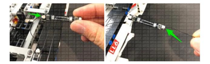
Using it's adhesive backing, stick the Red Strip Light vertically onto the black technic bar in the below position. Ensure the 5cm Connecting Cable in between is stretched out to prevent it from dangling down.
