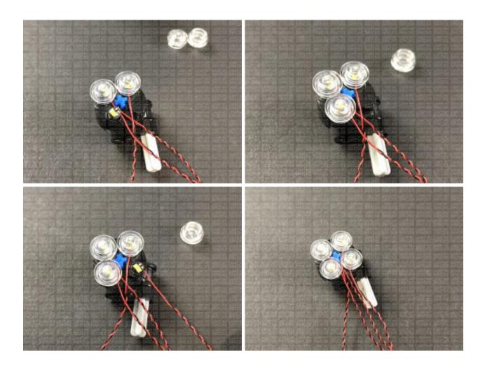
3.) Bring the four Bit Light cables together at the bottom of the headlight
