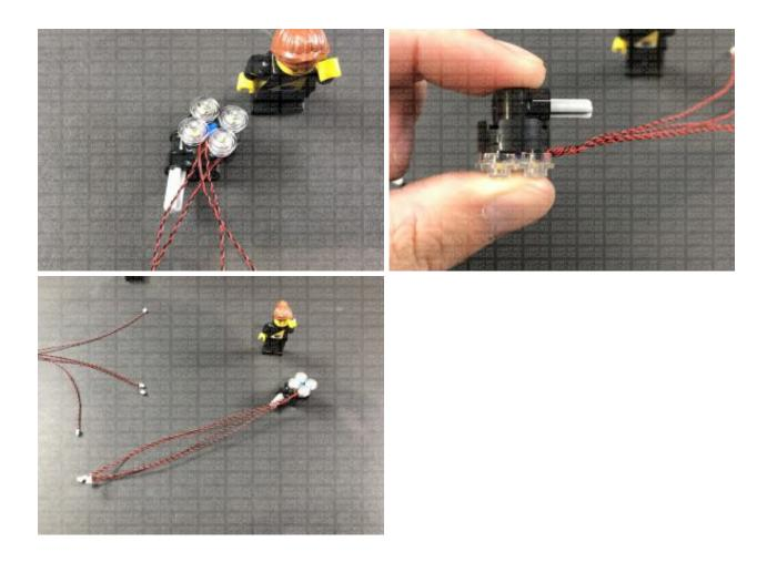
**5.)** Take the **12-Port Expansion Board** and connect all the lights from the two headlight sections to it. Take your AA Battery Pack and insert 3x new AA Batteries to it. Connect the battery pack cable to the expansion board, then turn it ON to test the 8 lights from the headlights are working OK.
