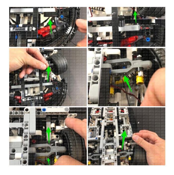
Thread the cable underneath the light grey technic bar, then bring it back over again and thread it through the technic bar hole towards the left. Ensure you tighten the cable as you pull it out from the other side.
