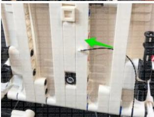
Connect the cable to a White Strip Light, then using it's adhesive backing, stick the strip light underneath the roof in the following position:
