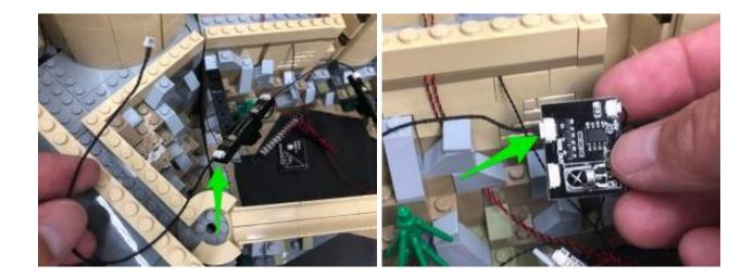
Lastly, ensure the RGB Board is facing the correct way up so that the IR sensor is visible and in line of sight to the remote control we will use to control it.
