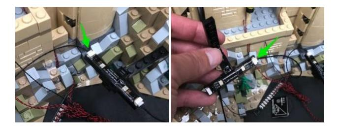
Connect the spot light to the below position to allow it to project up onto the large main tower of the castle.
