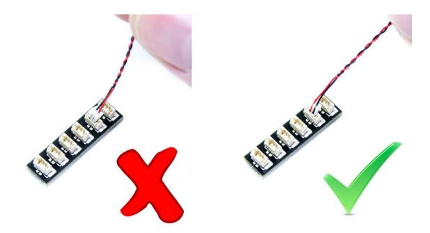
Incorrectly inserting the connector can can result in bent pins inside the port or possible overheating of the expansion board when connected.
