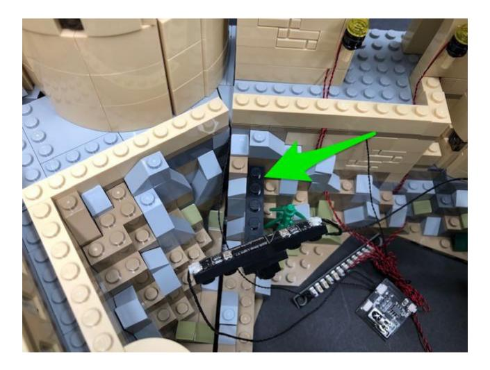
**71.)** Take the remaining **RGB 15cm Connecting Cable** and connect it to the right port on the upper spot light we just installed then connect the other side of the cable to one of the OUT ports on the RGB Board.
