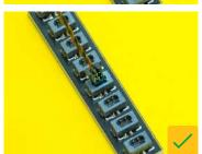
Not only will a light connected to the damaged port not work, but if the pins inside the port are bent to a point they are touching each other, this can result in all other lights in the system to stop working. This is a short circuit.
