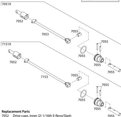
Drive cups, inner (2) 1/16th E-Revo/Slash (steel constant-velocity driveshafts)
