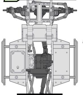
The Enduro drivetrain is designed to suit a variety of applications. The transmission can be rotated to allow for a more forward bias weight distribution, different motor rotational directions, and possible dig unit installations.
