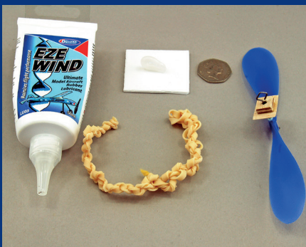
Pre-tensioned rubber showing just how much is needed for a 6-gram motor. Eze Wind was used as a lubricant.
