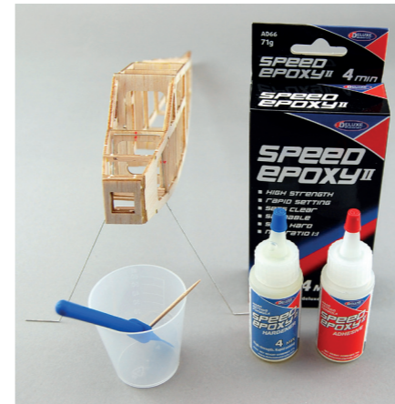
Speed Epoxy was used to stick the wire undercarriage to the Sparrowhawk.
