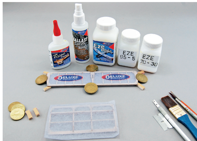
Support the airframe once first doped and after every Eze Dope coat thereafter. Coins make good weights.
