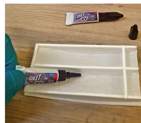
Above & above right: Rokat UV is foam safe. But use no more than is needed to tack a joint as a small amount of heat is generated as it sets. Depending on the foam thickness the UV torch is still effective when shining through it.
