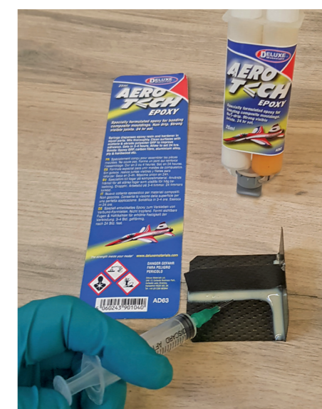
Left & above: Fabrication of small bulkheads using composites such as carbon sheet can be tricky, so a spot of Rokat UV is ideal for tacking composite parts in just the right place. Aero-Tech epoxy is solely designed for bonding composite materials such as carbon fibre sheet. With the bulkhead tacked in place using Rokat UV the epoxy can now be easily applied.
