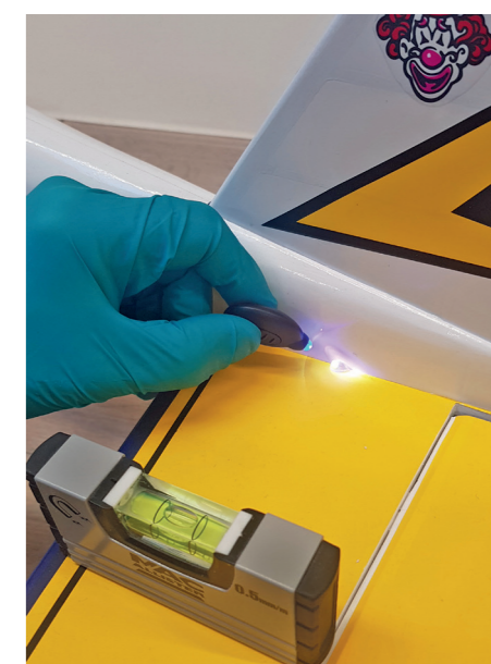
Rokat UV is ideal for joints that need a precise cure on demand, like this tailplane that needs to be held in careful alignment while the final glue joint cures. Here we are setting the tailplane in just the right place with a small spot of UV before securing the joint with Aero-Tech epoxy.
