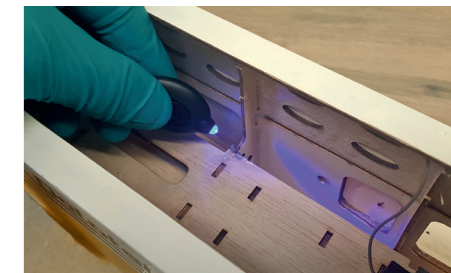
Rokat UV is also ideal for tacking wood. Here is a servo tray that needs seating in just the right position. You only need to apply a small drop before using the torch.
