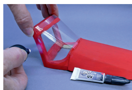
Rokat UV saves time when attaching clear canopies, which can be tricky to hold in just the right place. Just apply the glue and light.
