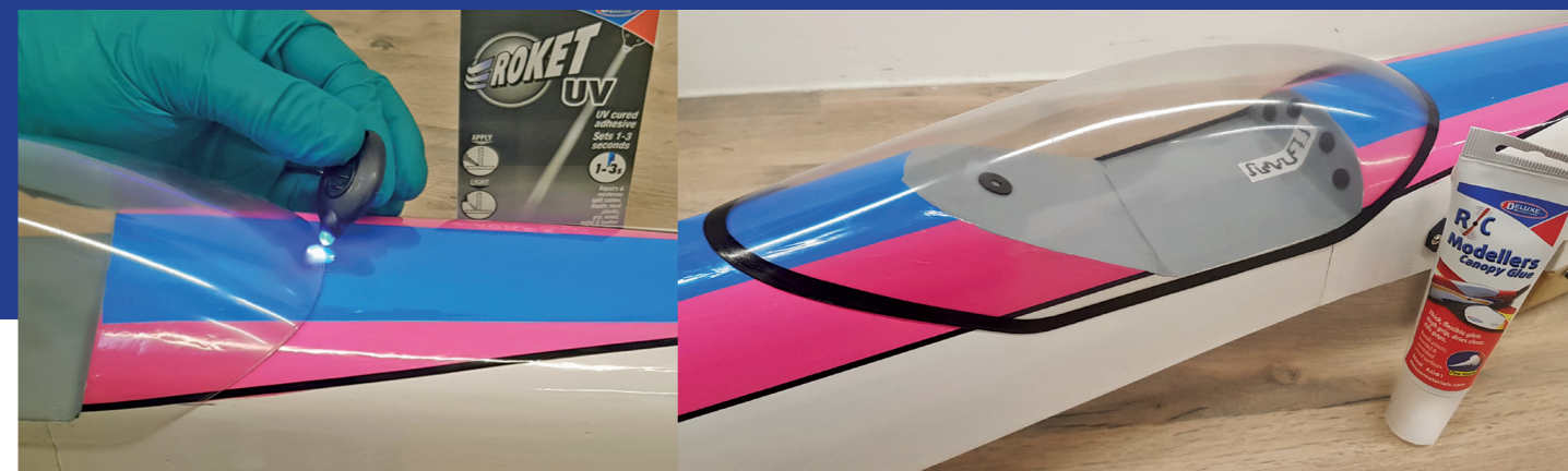
Here we are lightly tacking a carefully cut canopy in place prior to a final application of R/C Modellers Canopy glue. After the canopy glue was set, we taped up the joint.
