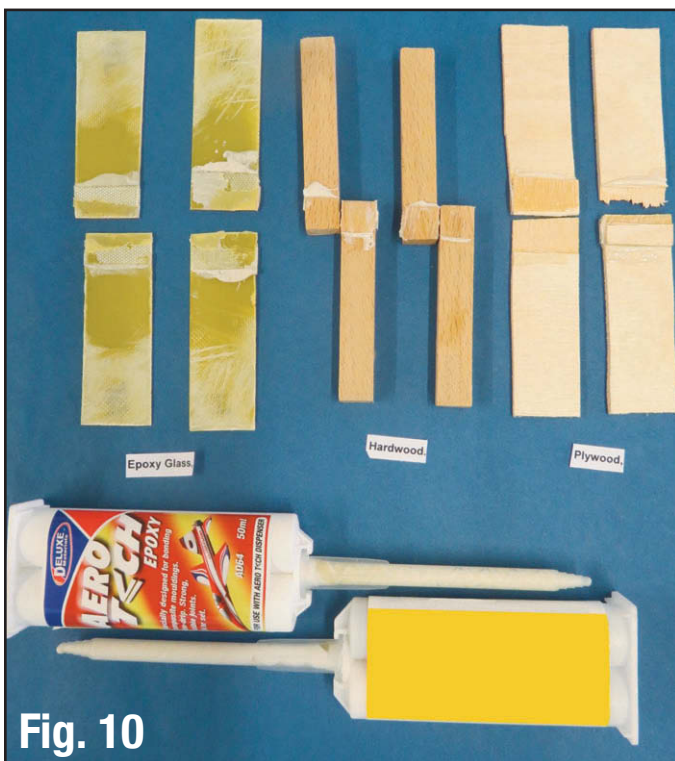
Results of epoxy glue tensometer tests newtons/ mm 2 : AeroT<ch versus competitor epoxy
