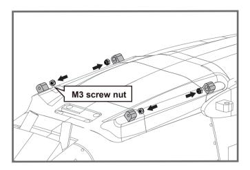
2. With the fuselage inverted, install the landing gear assembly and retainer then secure it with screws as shown in the diagram.
