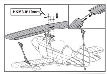
4. Once both wing halves are aligned, push the interplane strut rearwards to lock the structure.
