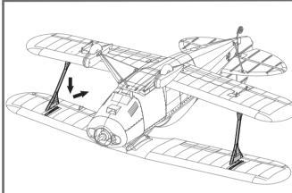
5. Connect the aileron pushrods between the upper and lower wings as shown in the diagram.
