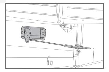
2. Install the pushrod to the control horn on the horizontal stabilizer as shown.
