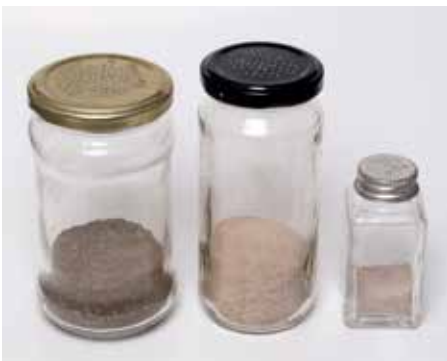
I used these homemade shakers as dirt applicators. I drilled the small holes in the lids, and the smallest applicator has smaller holes for applying very fine dirt.
