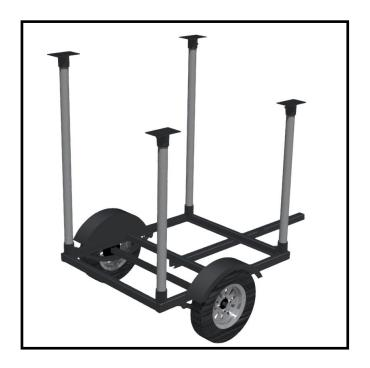
4. Place the 8ft long pipes on top of both brackets. Insert U-bolts and tighten the U-bolts. You may need a buddy for this step.
