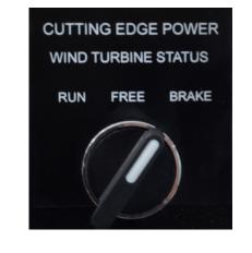
3. Set the brake switch to the "Brake" position
