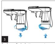
Replace cylinder bottom cover to enclose 3 oz cylinder –leave it open if using a 14.5oz (60L) cylinder, or sitting the unit onto the optional accessory stand for counter-top use.
