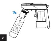
Slide out the Fizz Infuser with bottle again – gently shake the carbonated bottle before release. This will increase absorption of CO2 into the beverage.
