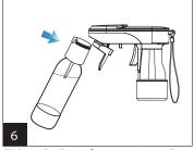
Slide in the Fizz Infuser – again, make sure the white plastic tip is not blocking the way. Push the Fizz Infuser and adapter to carbonating position (perpendicular to the frame).
