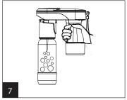
Pull the Trigger to carbonate – normally 2 - 3 times at one second each time. Maximum carbonation is reached if you hear a discharge whooshing sound and pressure release.
