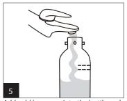
Add cold beverage into the bottle and connect it to Fizz Infuser – No hot or pulp liquids. Fill up to the Max. fill line. Connect both by holding the bottle and turning the Fizz Infuser clock-wise a quarter turn to lock.
