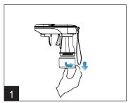
Remove the cylinder bottom coverremove the Pin Protector inside (For first time use only. Only on some models)
