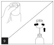
Release pressure – Lift the Slow Release tab and Fast Release button to discharge pressure. If the foam level is too high, let bottle set for awhile before discharging. To be safe, always finalize the pressure release process by depressing the blue Fast Release button.
