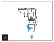
Install CO2 cylinder – remove the seal for new cylinder, insert threaded part into unit receptacle and hand-tighten.
