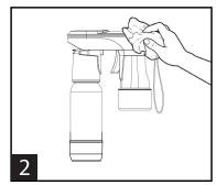
To clean the Spritzer Frame, wipe with a damp cloth. Do not immerse the Frame unit in water. Do not use any solvents or abrasive cleaners, since this could damage the surface.
