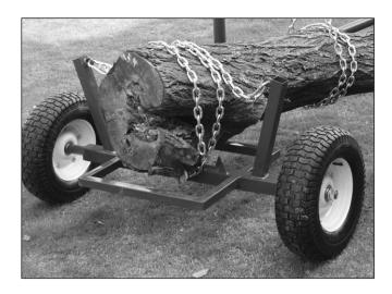
**Note**: Logs will be easier to move and stay mud-free with less snagging if you use the Rear Log Holder (#27) to hold the logs. However, if the transporting distance is short, or the log is not very large, you can use the log arch and holder alone to hold and skid the log.
