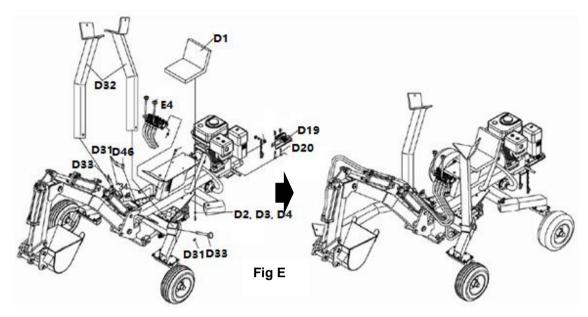
Note: The Swivel Safe Pin (D46) is a safety Pin. Remove it before using the machine and insert it when you want remove.
