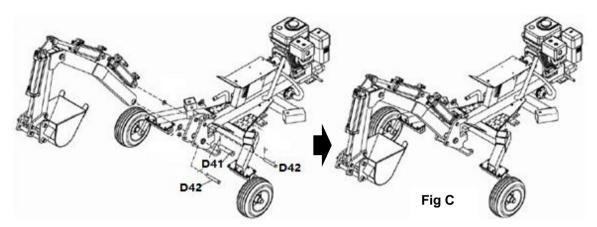
Note: The Pin (D41) is a safety Pin. Remove it before using the machine and insert it when you want remove.
