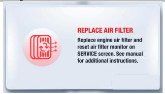
The engine air filter has reached the end of its life. Replace it to ensure proper operation of the generator. See engine owner's manual for details. After completion, reset the air filter change monitor on the service screen using below sequence:
