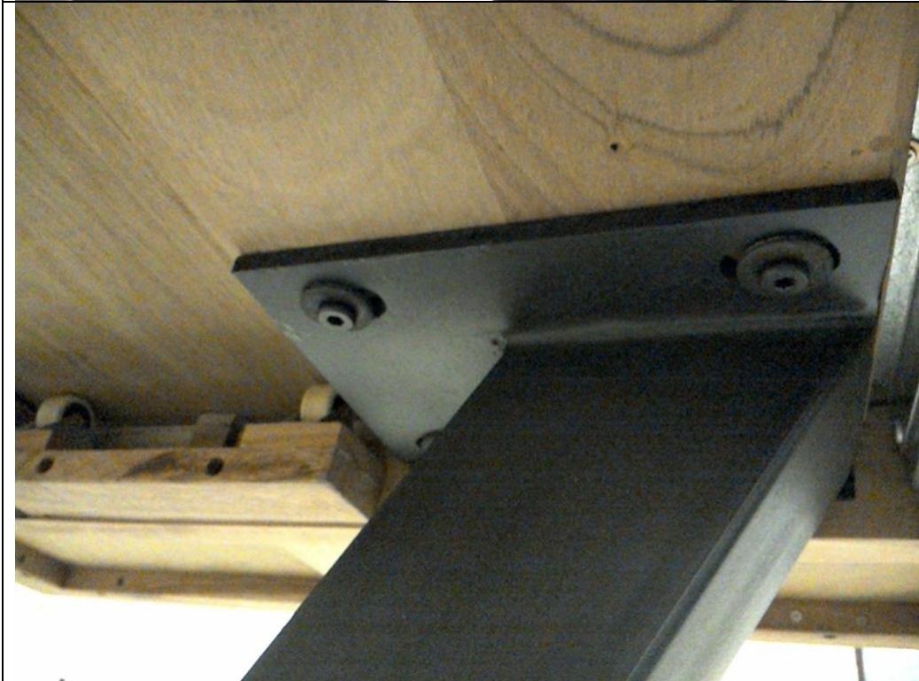
Bolts and washers. Holes are oval for adjustment of legs.
