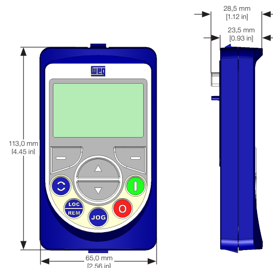
Figure A.1: Dimension drawing of the remote HMI serial HMI-01 Figura A.1: Dimensional de la HMI remota serial HMI-01 Figura A.1: Dimensional da HMI remota serial HMI-01
