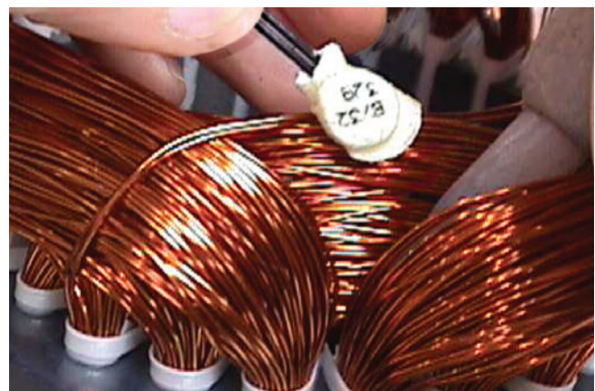
Figure 7.6 - Thermostat installation in the winding
