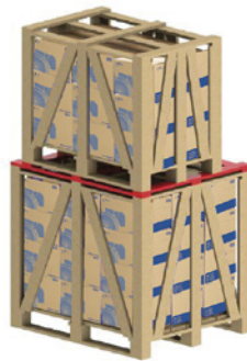
Figure 28 - Use of additional battens for stacking
