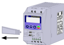
(a) Removal of front cover (a) Remoción de la tapa frontal (a) Remoção da tampa frontal
