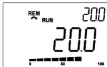
Figure 19.21: Example of HMI in the monitoring mode for the PID2 Controller function
