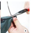
7. Using a heavy duty stapler (a regular stapler will not be sufficient for Manual shift rings, but would be fine for most DSG/Auto Rings), Periodically staple the boot to the trim ring like the factory boot. This step is optional as the adhesive is strong enough to hold the boot in place without staples.
