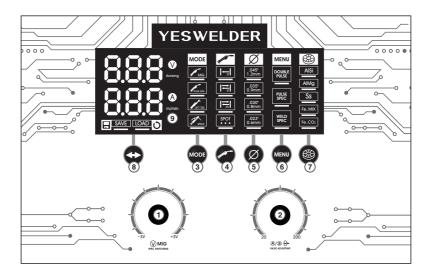
Function / Voltage Adjustment / Gas Checking Knob: Permits selecting Gas Pre-Flow, Post-Flow, Inductance, Rin, Hot start, Burn back time, Spot time in MIG and Pulsed MIG Mode, Synergy or Manual MIG in MIG Mode, Pulse / Double-Pulse Pulsed MIG Mode, IBS, FRQ, Duty cycle in Double-Pulse MIG Mode, Arc force, Hot start, VRD, and Anti-stick in Stick Mode. Permits selecting output voltage (fine-adjusting voltage in synergic mode).
