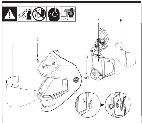
A Never use the auto-darkening lens without the inside and outside lens covers properly installed. Welding spatter will damage the auto-darkening lens and void the warranty.
