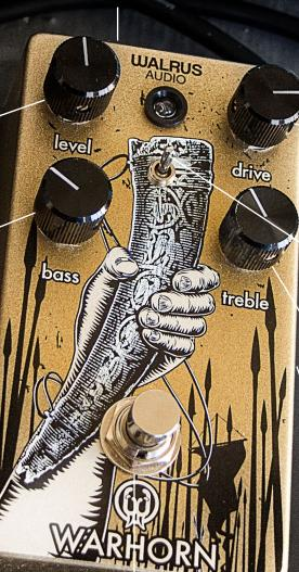
**DRIVE** – Adjusts how hard your guitar signal is clipped.
