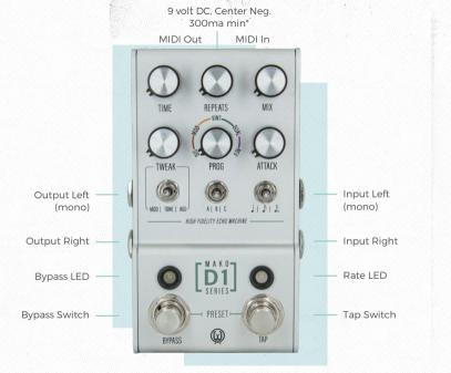
\*The use of an isolated power supply is recommended for powering all Walrus Audio Pedals.
