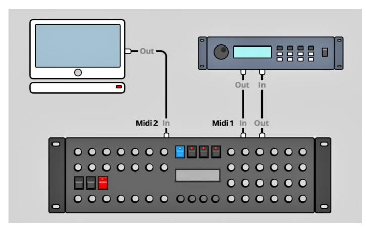
Both jacks of Midi 1 connect the Programmer with your synth in a loop. This seems unconventional but it is necessary: the Synth Programmer must hold the same patch data in it's memory as your Microwave. This data exchange runs through **MIDI 1 IN** / **OUT**.
