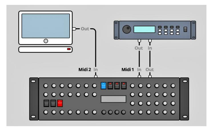
Both jacks of Midi 1 connect the Programmer with your synth in a loop. This seems unconventional but it is necessary: the Synth Programmer must hold the same patch data in it's memory as your MKS-80. This data exchange runs through **MIDI 1 IN** / **OUT**.
