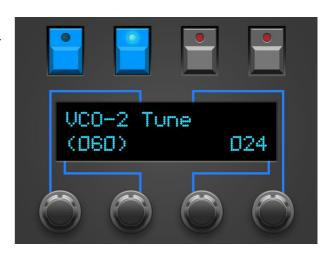
You can finetune the value of the currently active parameter with encoder 3. (Why encoder 3? Because the line printed on the faceplate leads from encoder 3 to the lower right corner of the display)
