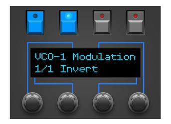
Each time you move a pot, the upper left display position shows the associated parameter group. For example you turn the knob for 'VCO-2 Tune', the upper left of the display shows 'VCO2'. If the para group is printed in CAPITALS, there is at least one sub parameter. The para group "Xmod" therefore does not offer a sub parameter. You reach sub parameters by moving encoder 1 or 4 one tick. Being in the sub group the enconders do the following:
