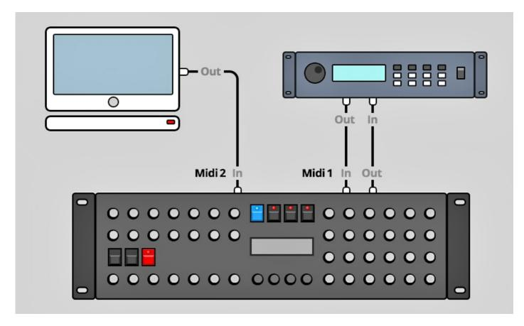
Both jacks of Midi 1 connect the Programmer with your synth in a loop. This seems unconventional but it is necessary: the Synth Programmer must hold the same patch data in it's memory as your Chroma. This data exchange runs through **MIDI 1 IN / OUT**.
