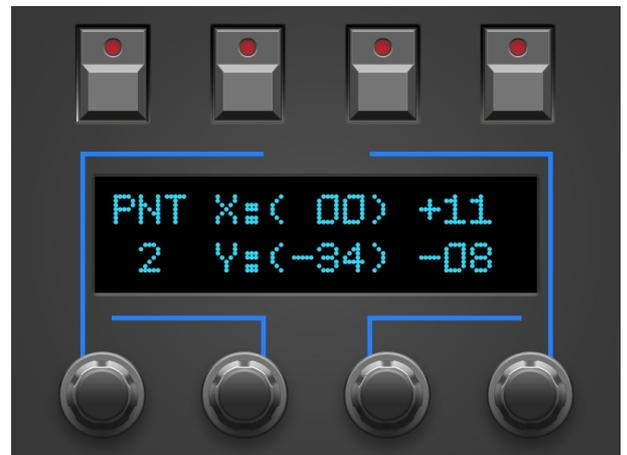
Now on the important part: right after touching one of the 10 WAVE ENV LEVEL knobs, the VS itself also jumps to the suitable WAVE ENV LEVEL display. You would like to set the levels with the joystick now, but ... in dependance of the parameter being active BEFORE touching one of the WAVE ENV LEVEL knobs, the joystick might refuse to set the WAVE LEVELS. Instead it does what it normally does – set the OSC mix for the currently held note.
