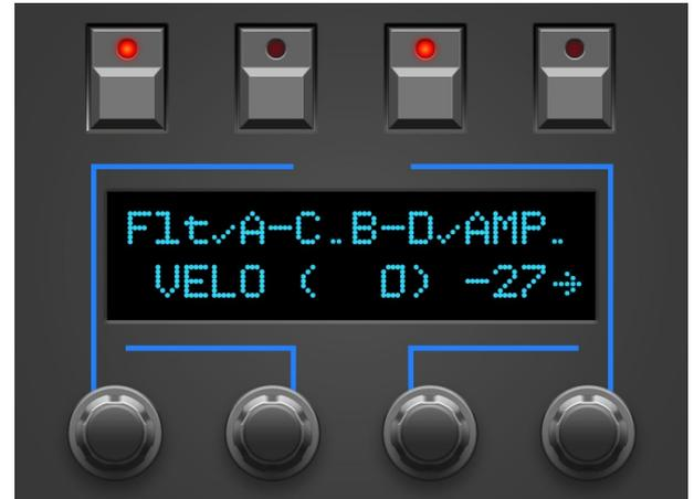
Line 2 also indicates the slotname (LFO1, PRESSURE ....) as well as the current modulation depth; as usual the program's original value in brackets and the currently set/edited value afterwards.
