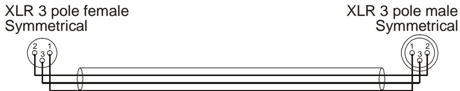
Used for connections between: microphone, amplifier, equalizer, loudspeaker-processor, limiter, etc and mixing panel.
