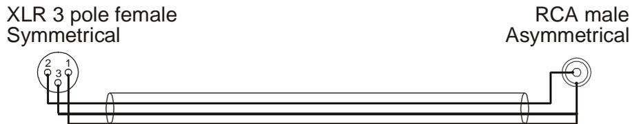
Used for connections between: professional CD-player, professional MD-player, sampler, effects-machine, etc and mixing panel.
