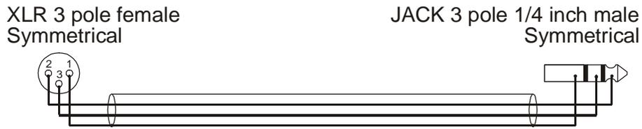
Used for connections between: microphone, amplifier, loudspeaker-processor, etc and mixing panel.
