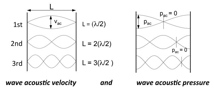
On a wall, the acoustic pressure is maximal and acoustic velocity minimal.
