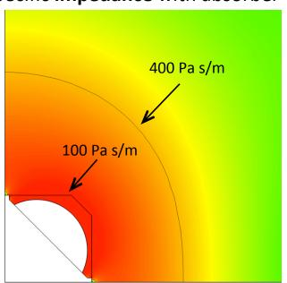
**Pressure structure** of the 1<sup>st</sup> mode with the absorber ON
