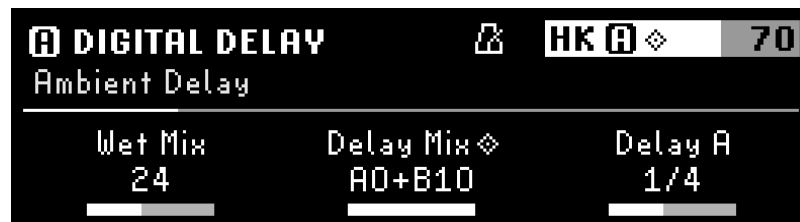
Fig. 6.31 A metronome icon will indicate that Tempo Sync has been enabled.
