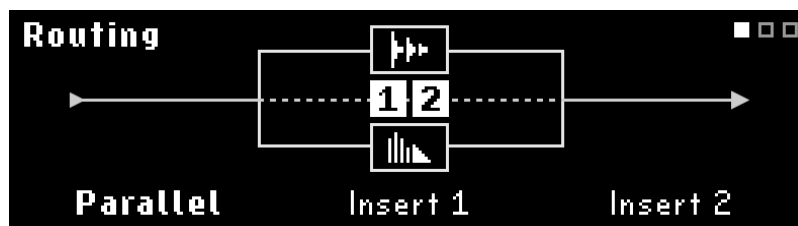
Fig. 6.10 Inserts 1 & 2 routed in Parallel with Preset A & B
