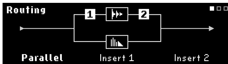
Fig. 6.11 Inserts 1 & 2 in Parallel, with Insert 1 pre-Preset A, and Insert 2 post-Preset B
