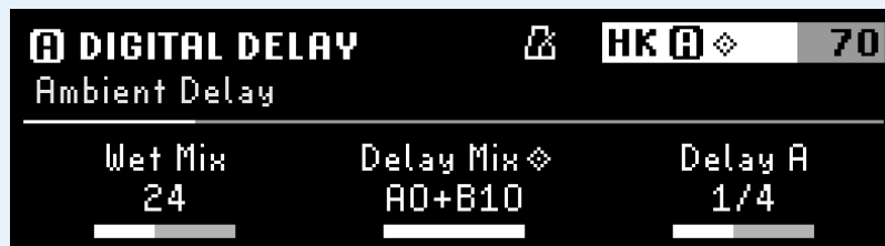
Fig. 8.3 A metronome icon will indicate that Tempo Sync has been enabled.
