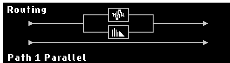
Fig. 6.17 Presets A &amp; B in Parallel on Path 1
