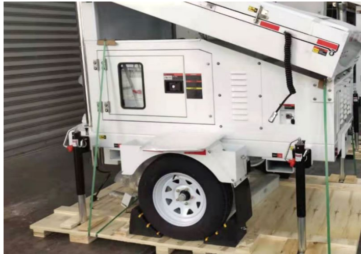
Forklift slots and removable tongue for easy and compact transport. Fits standard 463L pallet.
