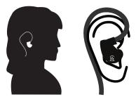
INSERT VEGA 2020 INTO YOUR EAR WITH THE CABLE EXITING FORWARD ALLOWING IT TO WRAP EASILY ABOVE AND BEHIND YOUR EAR. THE EARPHONES ARE 'HANDED' AND FIT EITHER YOUR LEFT OR RIGHT EAR. EACH EARPHONE HAS "L" OR "R" MOLDED INTO THE INTERIOR FACE OF THE EARPHONE'S BODY TO INDICATE THE SIDE.
