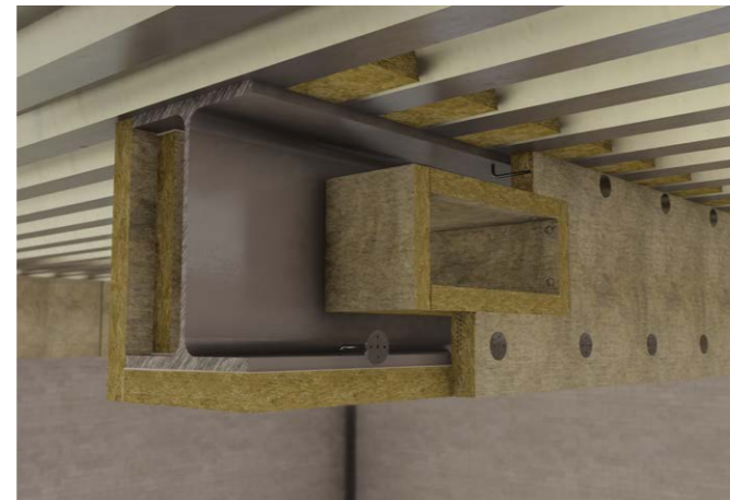
Figure 10 - Beam with square or rectangular holes (boxed protection - dry joints)
