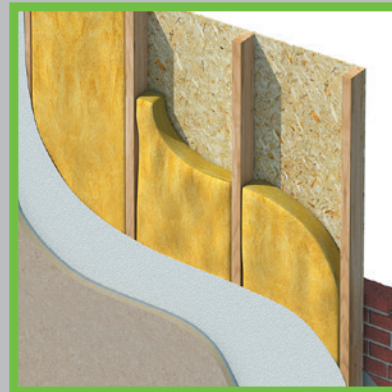
External Walls - Insulating between the timber studs
