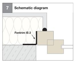
Window installed on the outside surface sealed airtight with Fentrim IS 2
