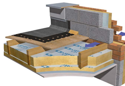
Flat roof: QR between & below joists
