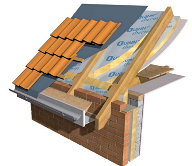
Pitched roof: QR between & below rafters
