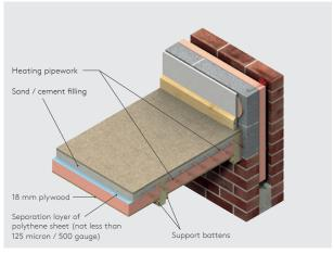
Figure 11: Intermittent Heating Applications - Suspended Timber Floor
