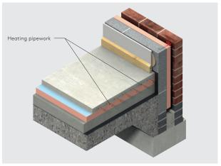
Figure 9: Intermittent Heating Applications - Below the Floor Screed
