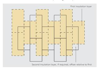
Figure 12: Offsetting of Multiple Insulation Layers
