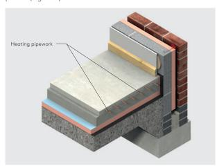
Figure 8: 24 Hour Heating Application - Below the Floor Slab
