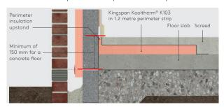
Figure 2: Perimeter Strip Masonry Floor Insulation
