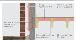
Figure 7: Complete Timber Floor Insulation
