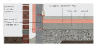
Figure 1: Complete Masonry Floor Insulation
