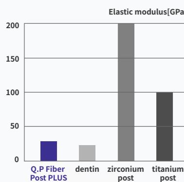
Elastic modulus similar to that of dentin helps to protect teeth without causing root canal fracture
