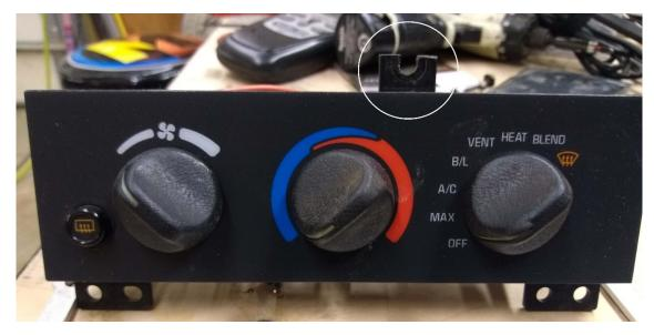
Step 6. Mount the A/C controls into the back of the new bracket with supplied screws. It should look like this when installed:
