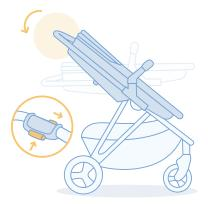
While holding the unlock tab, squeeze the front button on the front of the handlebar inward until you feel the stroller begin to fold, and push downward on the handle.
