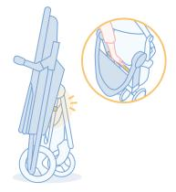
The stroller will fold until it is standing with the handlebar resting on the ground and the side latch "CLICKS". For a more compact fold, (don't worry about letting go for a second adjust the footrest downward to a 90 degree angle after you fold. If you need to move it once it's folded, just pick it up by the crossbar and you'll be on your way!
