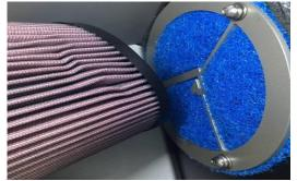
**9.** Install the air filter over inner MAF tube flange with included band clamp. Begin at the top of the flange and rotate the filter down and into place. Once fully seated on the MAF tube flange tighten the clamp to secure the filter.
