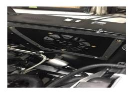
**6.** Mount the air box assembly to the inner fender apron panel using the 6 ½-inch stainless steel bolts with flat washers. Start all bolts by hand before tightening them evenly enough to compress the foam sealing gasket.
