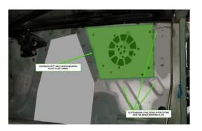
**4.** Clean surface with wax and grease remover and apply the foam air box seal to fender apron panel. Use the Rivnut positions to aid in aligning the foam seal into place.
